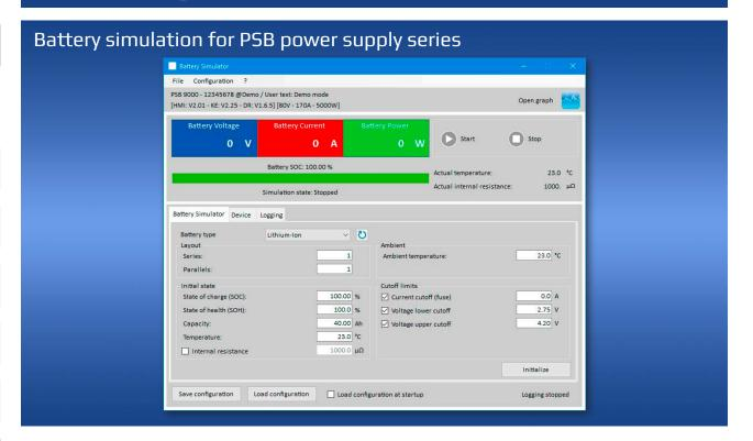
The **EA Battery Simulator** (EABS) is a Windows software with a graphical user interface, made to control all bidirectional devices of series EA-PSB 9000, EA-PSBE 9000, EA-PSB 10000 and EA-PSBE 10000. The bidirectional nature of these devices, which enables them work as energy source or sink, is essential for the simulation.
