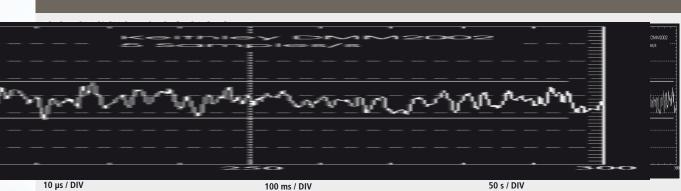
R1 EHS 8060: 6000 V/1 mA  $|V_{p,p} = 1.4 \text{ mV}$ R2 EHS 8060: 6000 V/0.1 mA  $|V_{p,p} = 0.4 \text{ mV}$ R3 Ground noise of the oscilloscope 0.8 mV **100 ms / DIV** EHS 8060: 6000 V/1 mA |  $V_{\rm p,p} = 11$  mV
