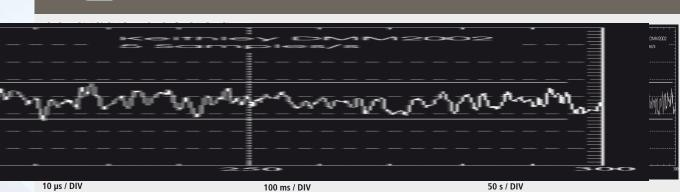
R1 EHS 8060: 6000 V/1 mA  $|V_{p,p}=1.4$  mV R2 EHS 8060: 6000 V/0.1 mA  $|V_{p,p}=0.4$  mV R3 Ground noise of the oscilloscope 0.8 mV
